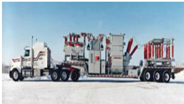
Figure 23 Mobile Substation and Transformer
